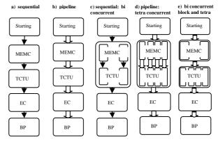
Figure 4: Explored MPEG-4 Configurations
